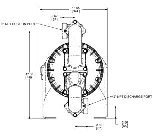
2" NPT(F) Suction and Discharge • <sup>3</sup>/<sub>4</sub>" NPT(F) Air Inlet Port • <sup>3</sup>/<sub>4</sub>" NPT(F) Air Exhaust Port (not shown)
