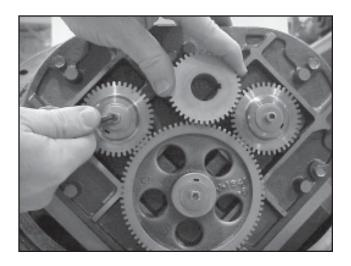
Keeping the spare displacement gear between the right rotor gear and blocking gear, use the allen wrench to loosen the screw of the right rotor gear assembly.
