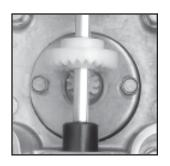
Adjuster drive gear engaged from the bottom.
