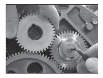
7. To loosen the screw of the blocking rotor gear, move the spare displacement rotor gear to between the left rotor gear and the blocking rotor gear to prevent the gears from moving.
