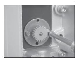
The packing gland may be taken apart by removing the retaining ring from the gear end of the assembly.
