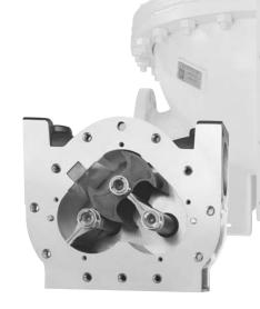
Liquid Controls' unique measuring chamber with no metal-to-metal contact minimizes wear and ensures precise and consistent measurements over a long service life.
