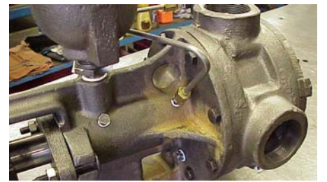
Figure 22, Bushing flush tube installed
