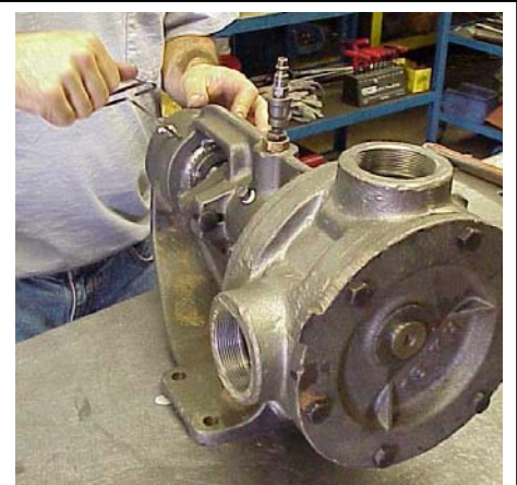
Figure 20, Tightening the set screws
