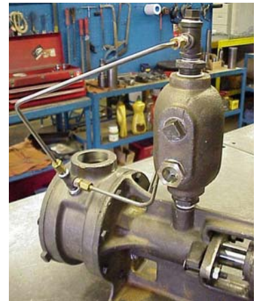
Figure 23, Reservoir and tubing installed
