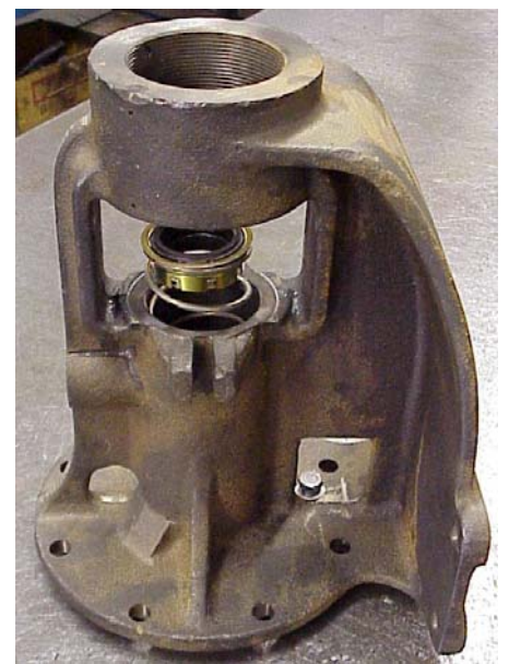
Figure 9, Installing the Seal
