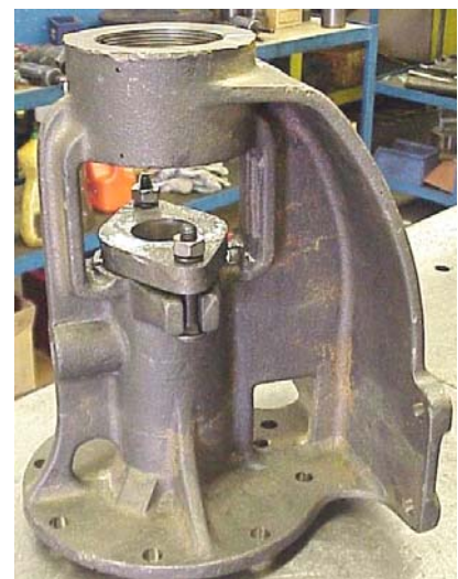
Figure 10, Outer seal seat retainer installed
