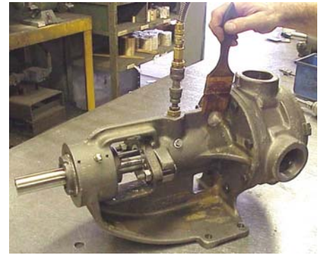
Figure 21, Testing the seal again
