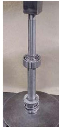
Figure 1: Pressing the bearing onto the Shaft
