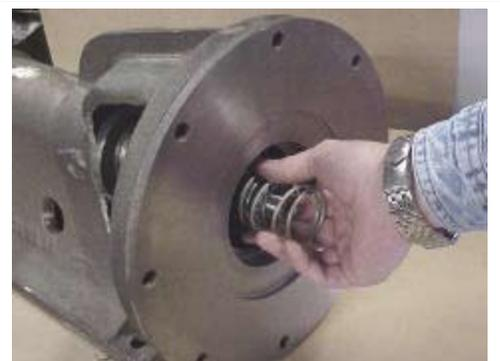
Figure 8, Installing the rotating seal
