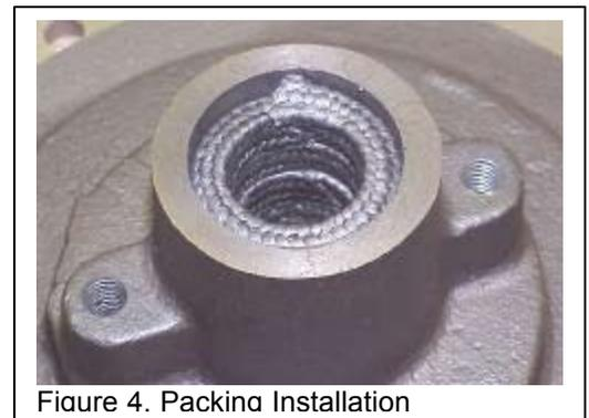
Figure 4. Packing Installation
