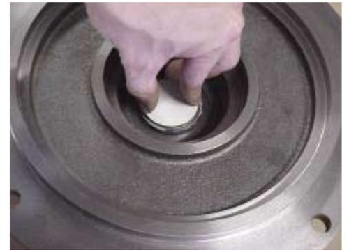
Figure 7, Installing the stationary seal element in the backplate
