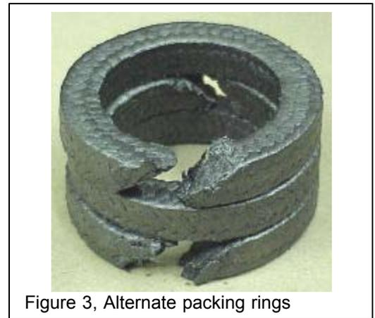
Figure 3, Alternate packing rings
