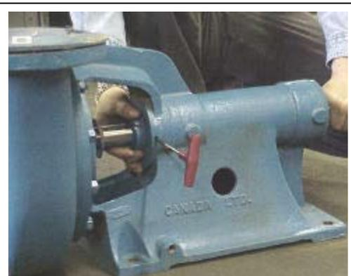
Figure 10, Adjusting the impeller
