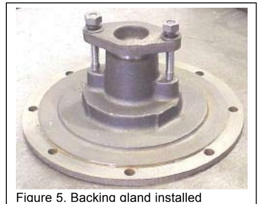
Figure 5. Backing gland installed
