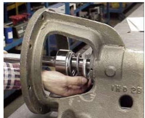
Figure 2: Installing the shaft assembly
